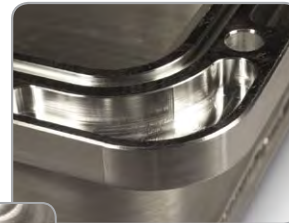
O-ring groove in fully machined pan rail
